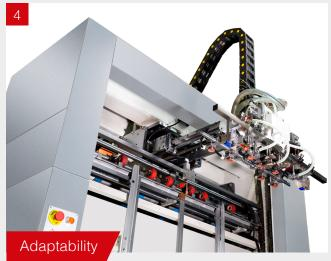
Servo motor driven suction feed head for top sheet, able to run large format.
