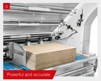
Substrate feeding with vacuum and servo motor intermittent driven system.
