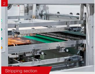
Includes upper and lower stripping frames with adjustable pins, supports, and telescopic bars for full manual setup. Also features an automatic window for easy access.
