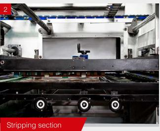
Quick format change with centering system and automatic support plate adjustment. Includes scrap remover, touchscreen control, micro-adjustment of the side guide, and safety systems.
