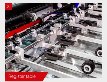
Register Table features 6 variable speed belts & anti-static stainless steel for better sheet control.
