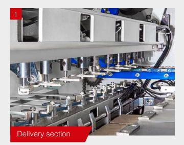
Two options to choose: Non-stop with motorized curtain and joggers for a squared stack or counted batch collection.
