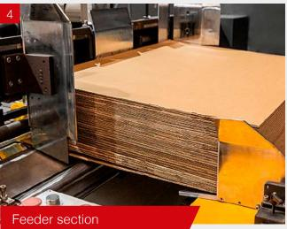
Feeder options include Bottom Belt, Lead Edge, and Anti-mark feeders with suction nozzles.
